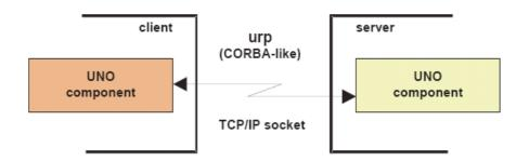
Figure 4: Communication between UNO components [Flat05].
