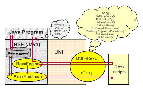
Figure 2: BSF interaction with ObjectRexx and Java, [Flat06].
